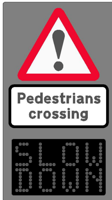
Fig1. Diag No. 562 with supplementary plate No.563. Vehicle activated panel with 'SLOW DOWN' text.
